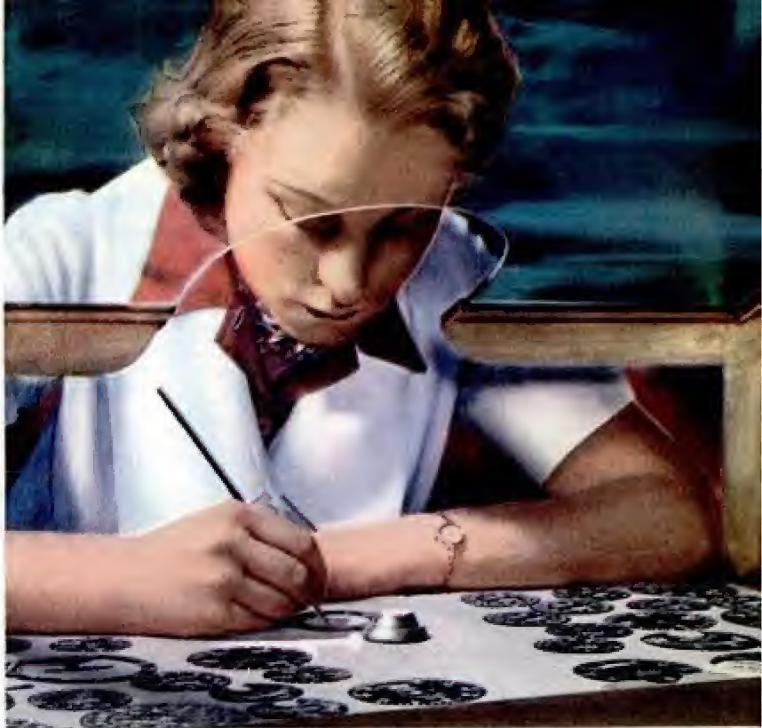
One important use of radium in war is in the making of luminous compounds. Here a worker paints aircraft instrument dials with a radium compound which makes them easily read in a dark cockpit
